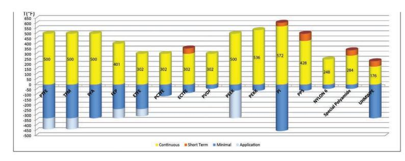
The graph indicates generic minimum and maximum temperatures for different polymers in Yellow and Blue respectively; the printed figured on each is the maximum continuous temperature possible. The extended range in Orange and Grey demonstrates that the polymers temperature envelope can be increased for specific applications and/or for short term use.
